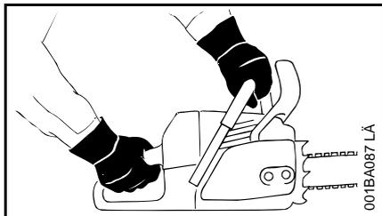
Your right hand should grip the rear handle. This also applies to left-handers. With your hands in this position, you can best oppose and absorb the push, pull and kickback forces of your saw without losing control (see section on reactive forces).
